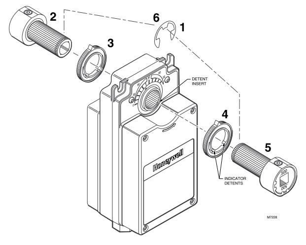
Fig. 3. Mounting hub to inside of actuator.
